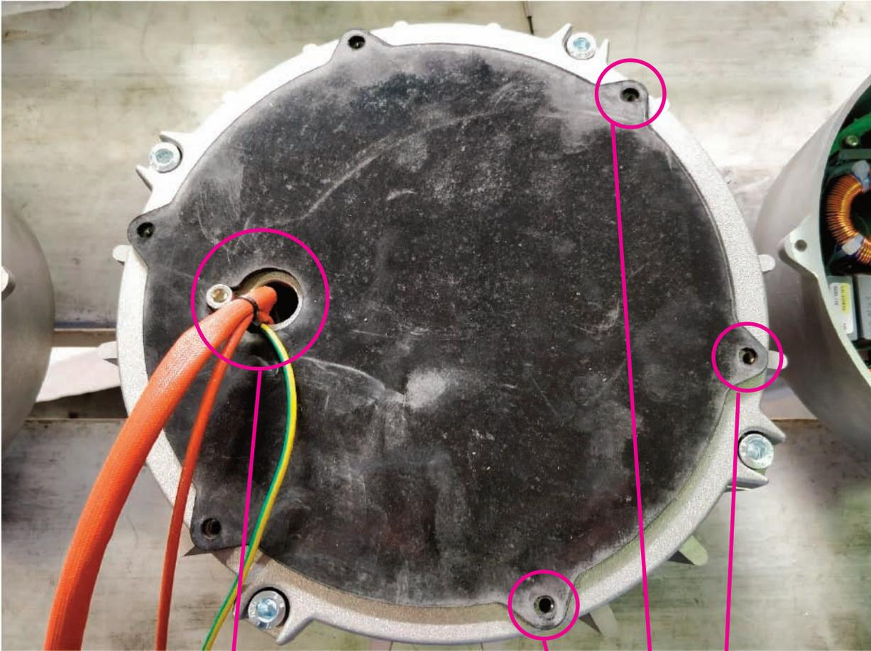
Position the motor part so that the motor cables are toward the left.
