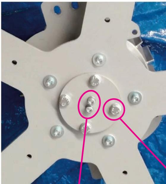
Remove the screws connecting the disc to the drive shaft
