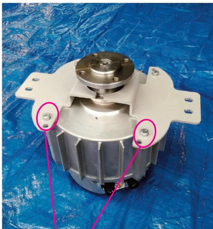
Remove the screws fixing the fall protection plate to the motor
