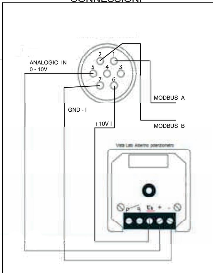
NB: It is necessary pull the A and B wires down to the control box for the Modbus connection, used for maintenance and diagnostic actions.
