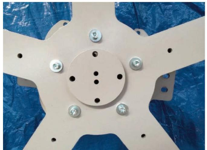
Remove the screws fixing the disc to the starwheel
