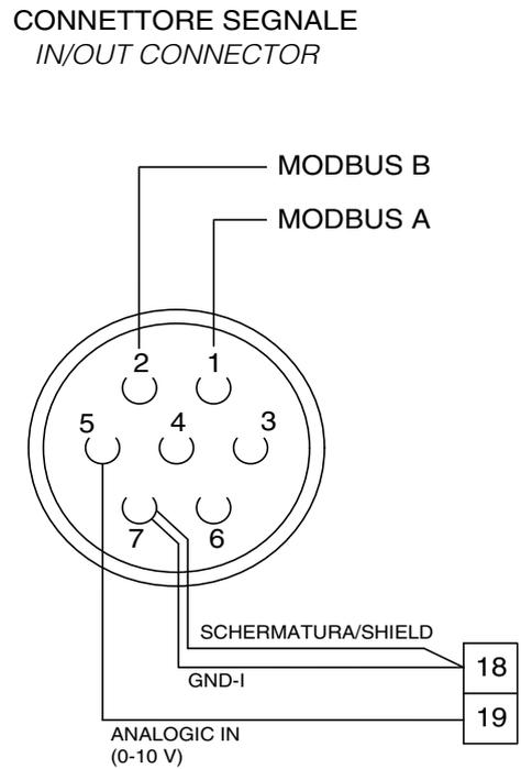
NB: It is necessary pull the A and B wires down to the control box for the Modbus connection, used for maintenance and diagnostic actions.
