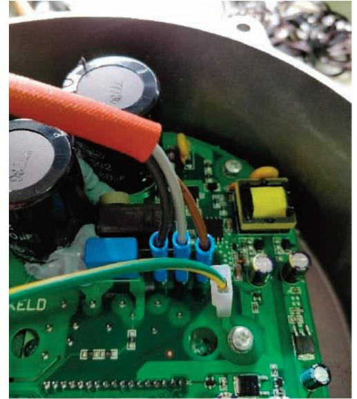
Insert the faston connectors on the motor phase electronics according to the following diagram:
