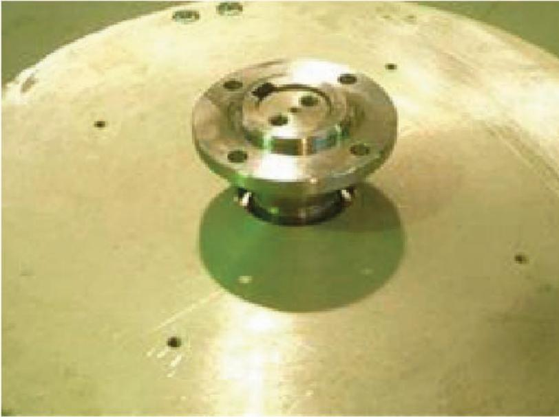
Slide off the fall protection plates and remove the hub from the shaft
