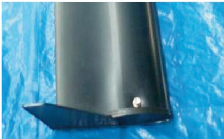
Unscrew the screw holding the plastic Winglet to the blade
