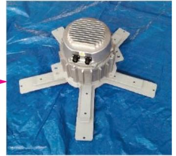
To assemble the bracket, you need to rotate the motor, resting it on the starwheel. Position the bracket over the motor so as to centre the holes on the fall protection plate.
