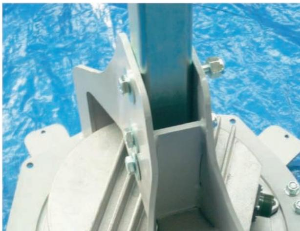
UNSCREW THE SCREWS FIXING THE ROD
