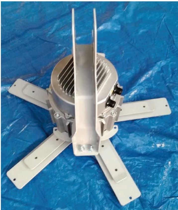
After having set the inverter motor on the ground, remove the bracket fixing screws.
